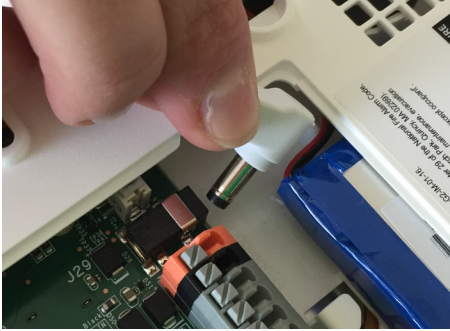
Plug in the power connector
