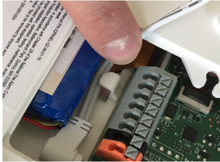
Route the wire behind the retainer clip
